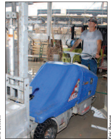
General Labor Foreman Tim Montalvo moves small material with the prime mover
